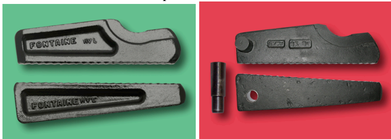
Caption: Numerous fleets have reported failures of non-genuine replacement parts installed in Fontaine No-Slack® fifth wheels, resulting in dropped trailers. The non-genuine components, including the failed wedge, are shown in the photo with the red background. Genuine Fontaine parts are shown in the photo with the green background.
