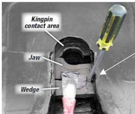
Separate the jaw and wedge with the screw driver here – grease the full length
