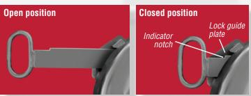
WARNING: If the pull handle indicator notch is not within the lock quide plate area, the lock is not properly closed and the secondary lock has not engaged.
