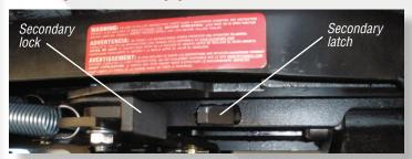
Inspect underneath the front of the top plate to verify that the secondary lock is properly engaged. When properly engaged, the secondary lock will be positioned inside the secondary latch toward the center of the fifth wheel (left-hand top plate shown in above photo).
