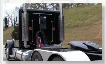
EASE OUT FROM UNDER THE TRAILER. Pull forward slowly until the fifth wheel clears the kingpin. Dump the air from the tractor suspension, and drive carefully away from under the trailer.
