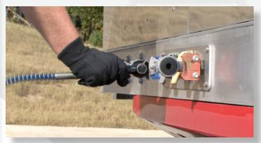
**DISCONNECT ALL CABLES.** Disconnect the air and electrical lines from the trailer.
