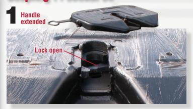
MAKE SURE HANDLE IS EXTENDED AND LOCK IS OPEN. When the handle is extended and the tips of the jaw and lockbar are visible in the throat of the fifth wheel, the lock is in the open position. If there is any debris (e.g. snow, ice or excessive grease) in the throat of the fifth wheel, it must be removed prior to coupling.
