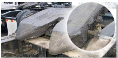
Over-lubrication is costly and causes excessive build-up on fifth wheel components leading to lost revenue.
