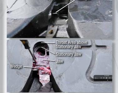
Separate the jaw and wedge with a screw driver and press the recommended lubricant between the serrated surfaces. Work the pull-handle back and forth to spread the lube over all surfaces. Also grease the Stationary Jaw and the Throat Area above the Stationary Jaw.
