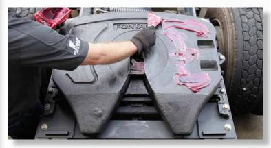
Lubricate the top plate surface with a thin layer of grease—leave area around jaw and wedge free of grease (skip this step for the 7000CC Clean Connect™ model).
