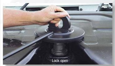
Insert a dimensionally correct test kingpin tool into the throat of the fifth wheel. Carefully push the kingpin in until the locking mechanism is activated. Keep your hands out of the fifth wheel throat.
