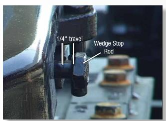
Check the travel of the wedge stop rod by pushing in on it. It should move in 1/4" with hand pressure and then spring back out. To obtain a proper setting, turn the wedge stop rod clockwise to reduce the gap and counter-clockwise to increase it. Adjust until the free travel is 1/4".
