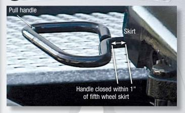
Verify that the pull handle is in the fully locked position (within 1" of the fifth wheel skirt).
