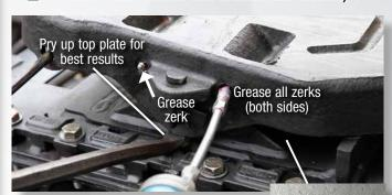
Grease the mounting brackets. Lift the top plate up with a pry bar to ensure grease gets to the top of the brackets. (Inspect mounting bracket base, and if "LUBE FREE" is cast into the bracket skip this step. These models have bracket liners and do
